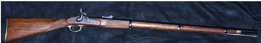
Whitworth .451 calibre muzzle-loading hexagonal-bore rifle
